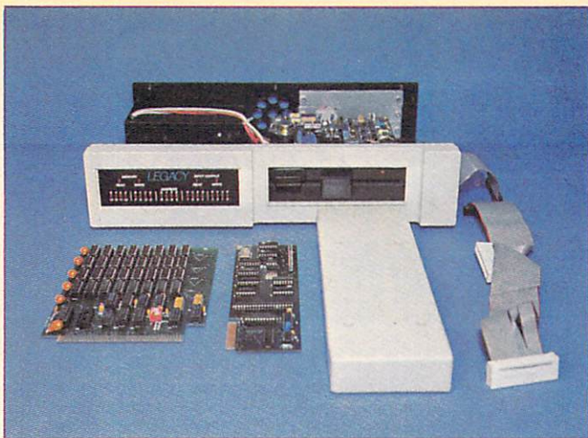
PHOTO 1: Everything shown here comes in the Legacy II system kit, with the exception of the fully populated memory card. The memory card is shown in the left foreground above.
